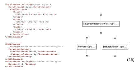
$\mathbb{C}_3$  is a symmetric monoidal category that refers to the category of CRCL commands. This is a category with one object per robot platform,  $R \in S^3$ , and arrows where arrows are fully parameterized CRCL commands.
