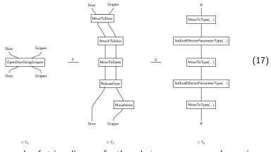
Full example of string diagram for the robot program: open door using gripper
