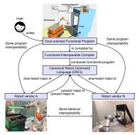
Figure: RoboCat framework consists of a goal-oriented functional programming environment, a functional interoperable compiler, and the mapping to the Canonical Robot Command Language (CRCL) and robot-specific APIs
